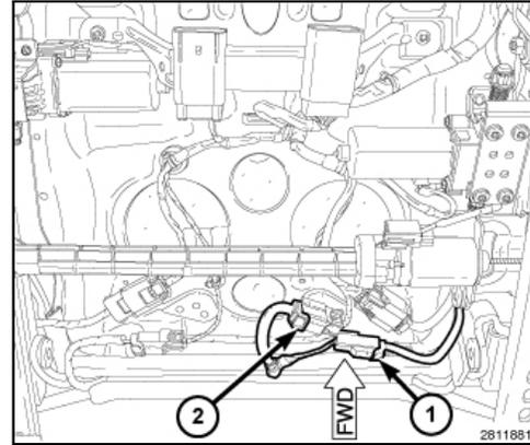
**NOTE:** When testing the heated seat elements for resistance, be certain to sit in the seat in question and move around the heating elements within the seat while testing. Moving the heating elements will help eliminate the possibility of an intermittent open in the element, which would only be evident in a certain position.
